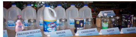
A display of the various industrial or household chemicals ingredients in hydraulic fracturing fluid.
